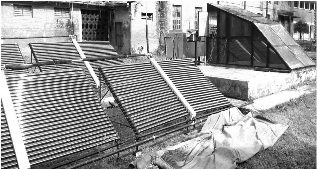
FRI PCM (Phase Change Material) based latest Solar kiln
