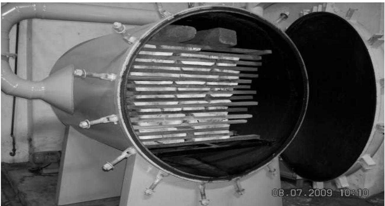
FRI convection heating based vacuum kiln
