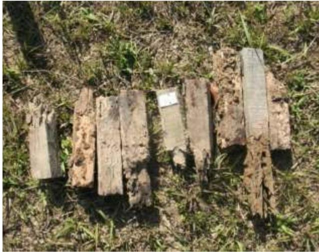
Natural durability test of imported timber in field
