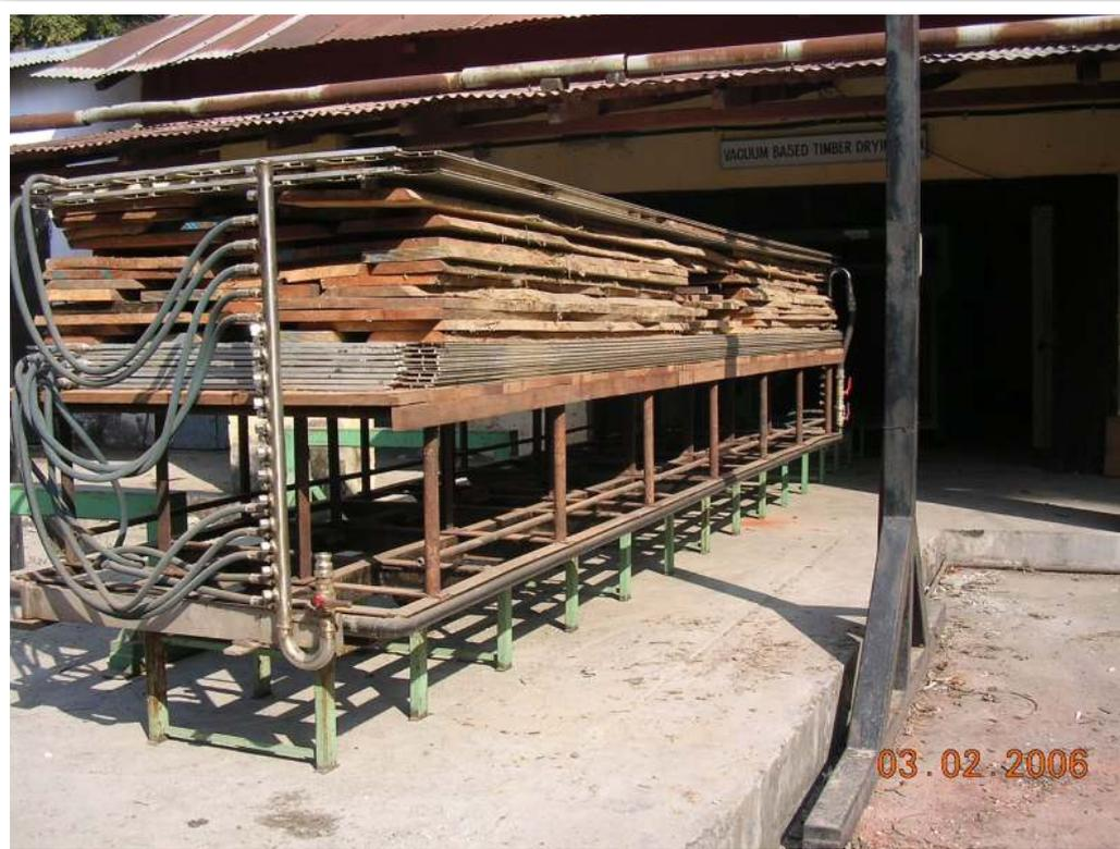
Timber stack ready to place inside the hot press type vacuum kiln
