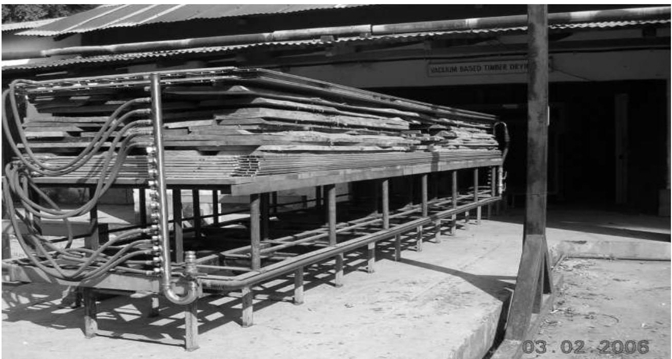
Timber stack ready for keeping inside the Hot press type vacuum kiln
